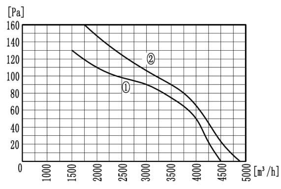
Curve 1: 50HZ Curve 2: 60HZ
